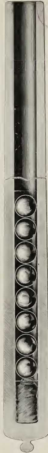
FIG. 66. SECTION OF BESSEMER STEEL GUN SUPPLIED TO THE BELGIAN GOVERNMENT, 1860
